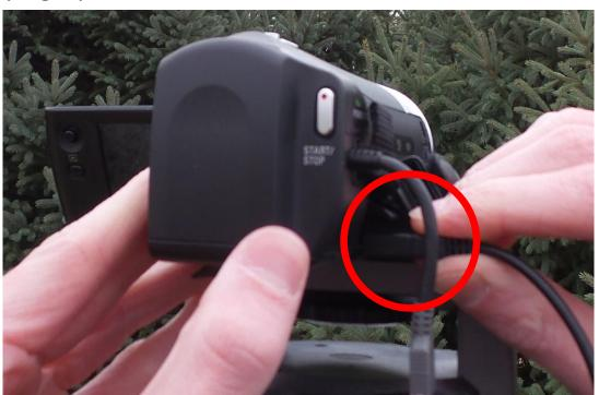
Step 7: Connecting HDMI Cable to Camera
