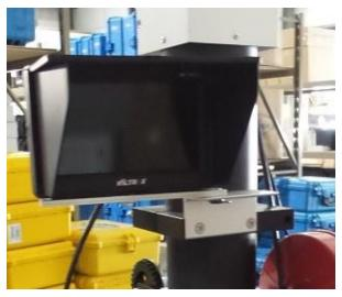
On the Tower, find the Monitor Attachment Plate. Insert the plate's mounting screw into the threaded receiver on the bottom of the monitor. Tighten securely.
