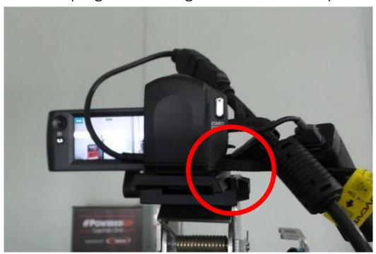
\*FRAGILE PLUG-IN\* On the right side of the camera toward the back, open the flap to expose the MultiPort plugin port. Plug the MultiPort cord into the MultiPort plugin port.
