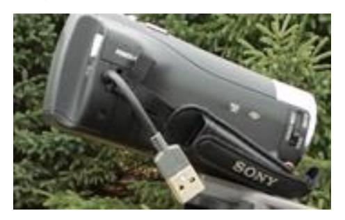
Plug the USB Charging plug into the Sideline Power External PowerPack Battery and let it hang
