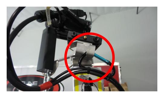
Step 6: Connecting Remote to Camera CAREFULLY plug in the Budget Remote's Multiport.
