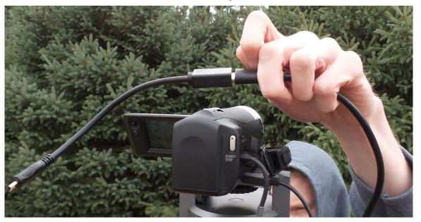
\*FRAGILE PLUG-IN\* Run HMDI cord through the camera's hand strap, and then up and over the camera. Then the Micro HDMI plug is inserted into the port we uncovered earlier on the LEFT SIDE of the camera.
