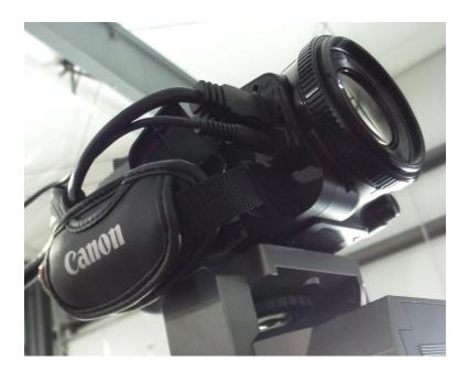
\*FRAGILE PLUG-IN\* On the right side of the camera open the flap to expose the plugin ports. Plug the LANC cord and MINI HDMI
