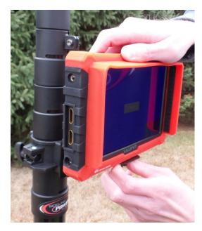
On the Tower, find the Monitor Attachment Plate. Insert the plate's mounting screw into the threaded receiver on the bottom of the monitor. Tighten securely.
