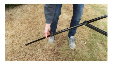
Keep the upper and lower tripod collar locking knobs loose until tower is situated a few inches above the ground. Try to maintain a 90° angle between the mast and leg supports.
