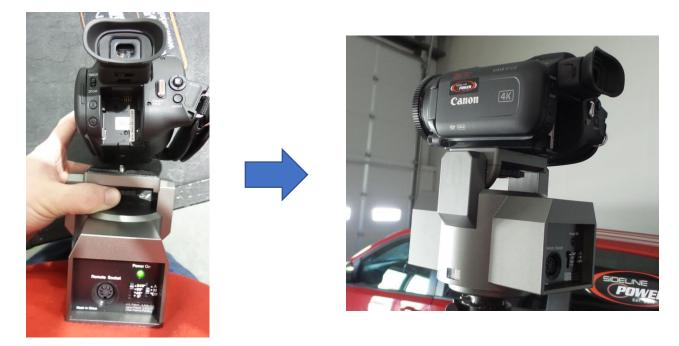
Pictures below show how the camera should be positioned on the Pan/Tilt Module.
