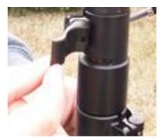
Once a mast section is raised to the desired height, close the quick release lever, locking the mast lock and securing the mast section in place. Use the BONGO Tie to secure the Remote Cable and HDMI cord bundle to the upper mast section.
