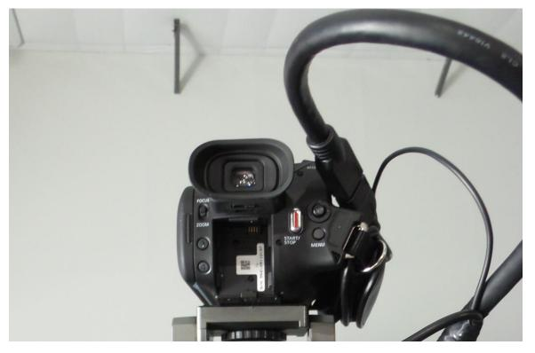
\*FRAGILE PLUG-IN\* Run HMDI cord through the camera's hand strap, and then up and over the camera. Then the Mini HDMI plug is inserted into the port we uncovered earlier on the RIGHT SIDE of the camera.
