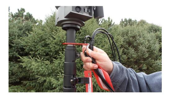
When connected, the carabiner should orient so the cord ends are pointing up toward the camera assembly.
