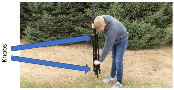
Spread the tripod legs outward by pulling the legs out and moving the upper and lower tripod collars.
