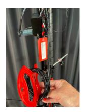
. Flip the quick release lock levers open for the mast sections and raise each section, one at a time, locking it into place at the desired height.
