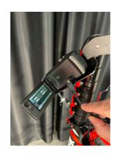
. Under the hand retention strap, locate the multiport reciever and plug in the multiport cord from the harness.
