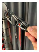
. Plug the micro HDMI adapter from the harness into the micro HDMI port on the camera.
