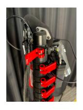
. Rotate the Top section of the tower so that the vertical part of the camera mounting plate is lined up with the manual pan/tilt handle.
