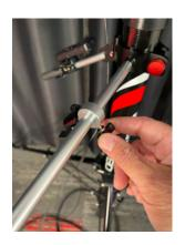
. Rotate the mount to the upright position and twist the locking knob clockwise to tighten.
