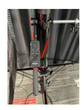
. Plug the multiport cable into the top of the camera remote.
