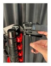
. Unlock the top quick release lever so the top section of the tower rotates freely.
