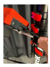
**38**. Twist the red tilt cable locking screw counter-clockwise to loosen.
