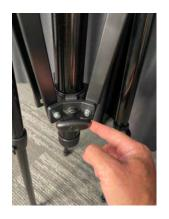
. Spread the tripod legs until the support braces are perpendicular to the tower mast.
