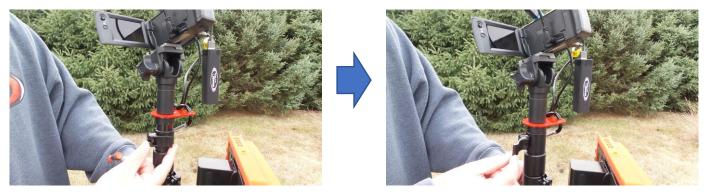
Once a mast section is raised to the desired height, close the quick release lever, locking the mast lock and securing the mast section in place.
