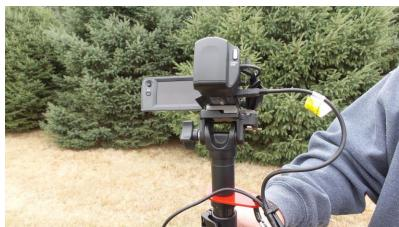
\*FRAGILE PLUG-IN\* On the right side of the camera toward the back, open the flap to expose the MultiPort plugin port. The MultiPort cord, has yellow tag attached to it. Plug the MultiPort cord into the MultiPort plugin port.
