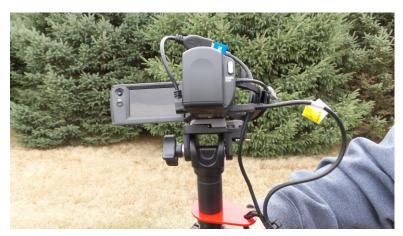
\*FRAGILE PLUG-IN\* Take HMDI cord w/ Micro-HDMI converter and route it over the top of the camera for increased slack. The Micro HDMI plug is inserted into the port we uncovered earlier on the LEFT SIDE of the camera.
