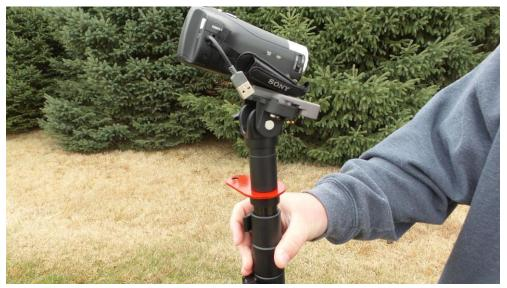
Looking at the rear of the camera, locate the integrated camera screen on the left side of the camera. Flip the camera screen open to 90 degrees to power on the camera. Open the the connections cover on the side of the camera body to reveal Micro HDMI port.
