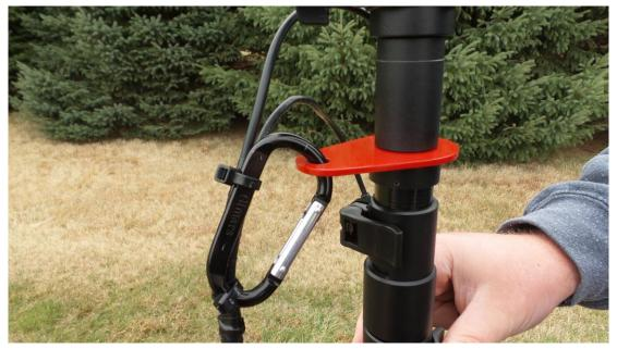
On the right side of the camera, remove the USB charging plug from its sheath on the camera retention strap.
