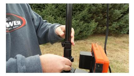
Continue this process until all mast sections have been extended and MonoPod is at desired height.
